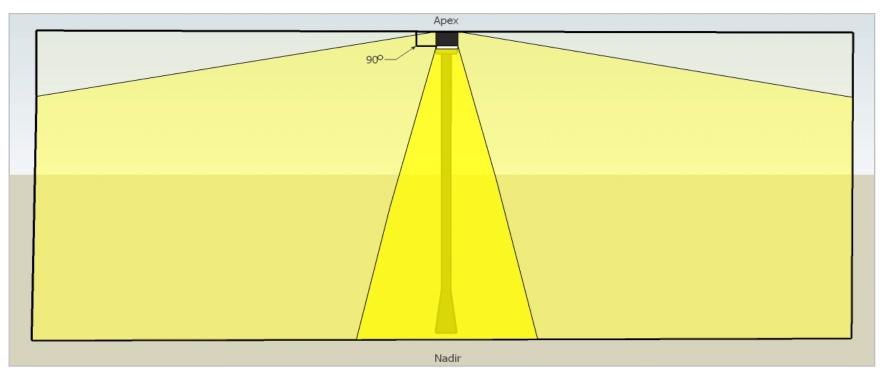
Figure 3: Full Cut-off Fixture
