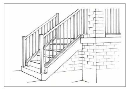
MASONRY VENEER SHALL BE APPLIED TO THE SIDE OF MAIN ENTRY STAIRS, WHERE MORE THAN 3 STEPS ARE REQUIRED.
