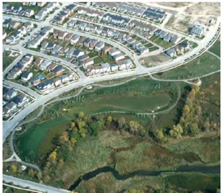
Where feasible, single-loaded roads adjacent to environmental areas promote visual and physical access.
