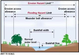
Figure 3.43 Erosion Hazard Limit in Confined System (left) where Toe of Valley Slope is < 15m from Watercourse (MNR, 2002); Compared to Erosion Hazard Limit for Unconfined System (right).
