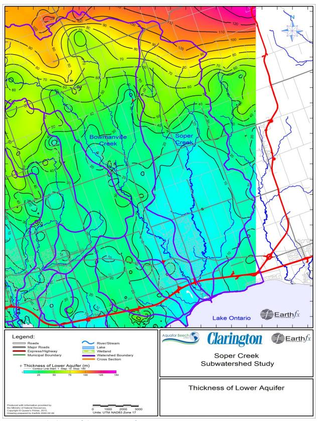
Figure 3.21: Thickness of the Lower Aquifer
