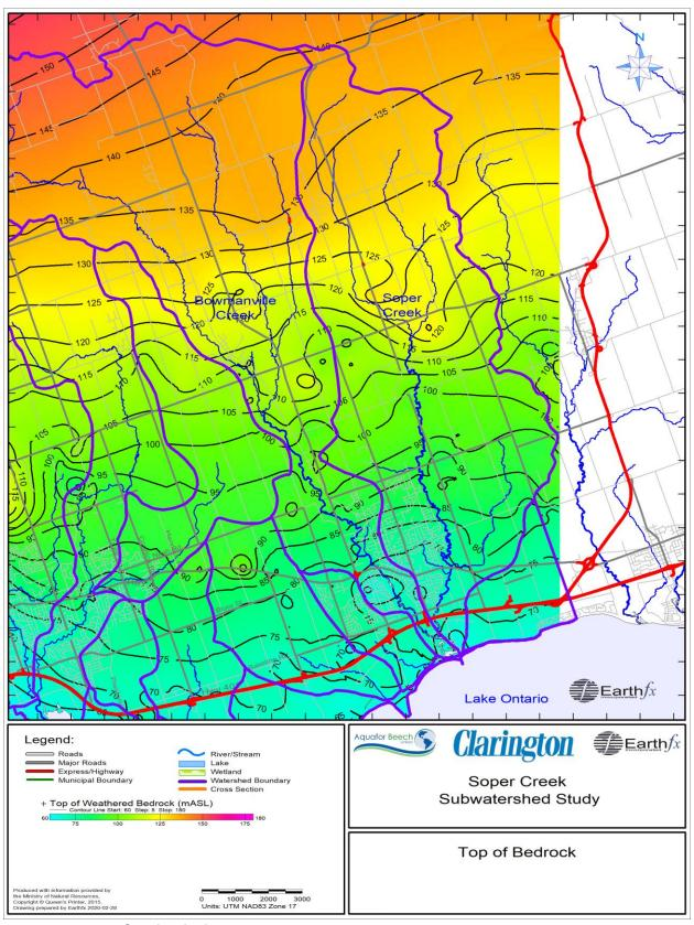
Figure 3.7: Top of Bedrock Elevation
