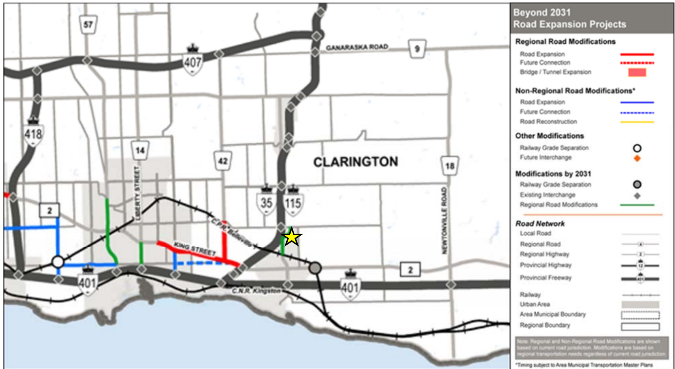
Figure 23: Durham Transportation Master Plan - Future Proposed Road Network Beyond 2031 Figure 15 Durham Transportation Master Plan - Future Proposed Road Network Beyond 2031
