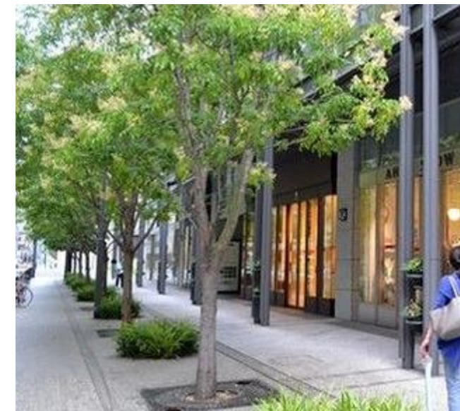
Street trees in tree grates planted and continuous pits
